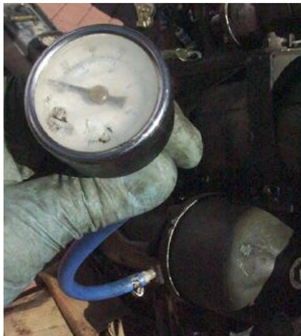
Pressure gauge attachment to front of oil filter
