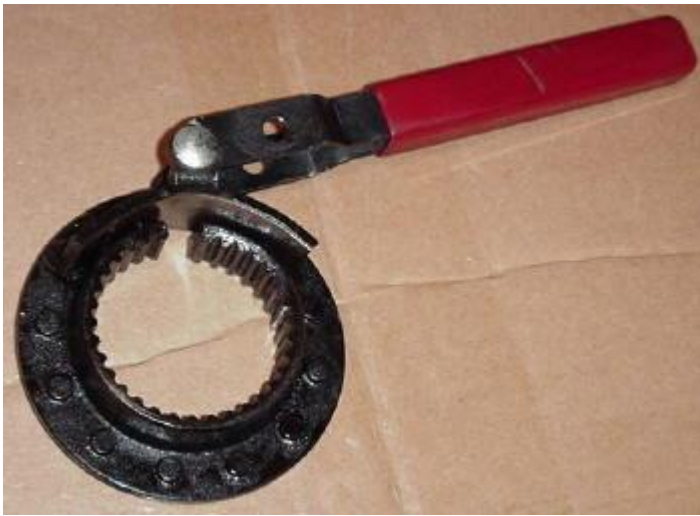
Manual trans clutch disk hub welded to a handle
