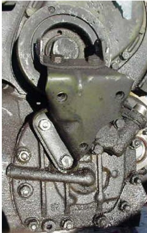
The Forward Clutch is behind the Governor Housing cover
