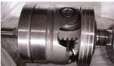
Top and reverse clutch assembly is removed
